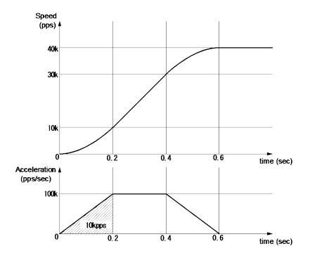
Fig. 2.2-13 Example of Partial S-curve Acceleration / Deceleration Driving
