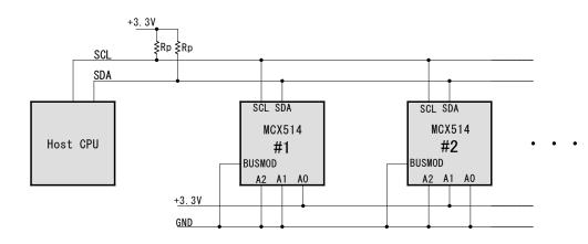
Fig. 4.1-1 The Connection Example of I<sup>2</sup>C Serial Bus
