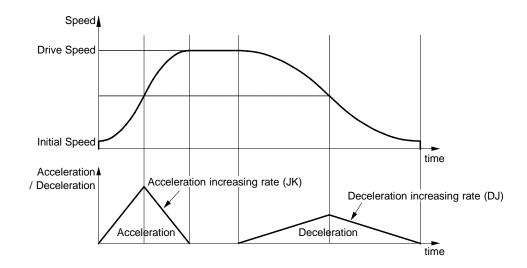
Fig. 2.2-14 Non-symmetry S-Curve Acceleration/Deceleration Driving
