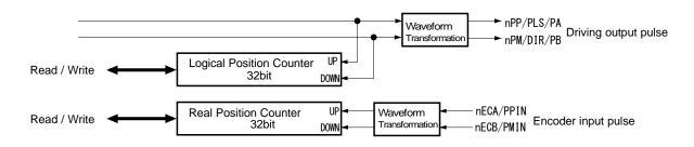
Fig. 2.3-1 Position Counter Functional Block Diagram
