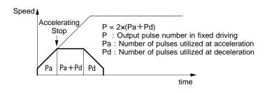
Fig. 2.2-5 Triangle Prevention of Linear Acceleration Driving
