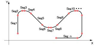
Fig. 1.1-3 Example of Continuous Interpolation
