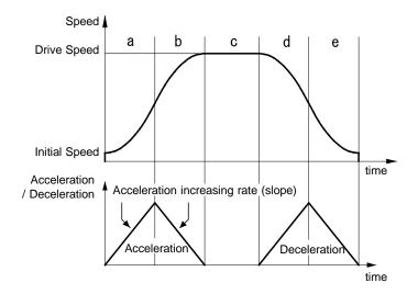
Fig. 2.2-8 S-curve Acceleration/Deceleration Driving (Symmetry)
