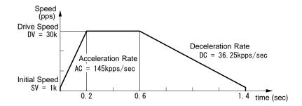
Fig. 2.2-7 Non-Symmetrical Linear Acceleration Driving (acceleration > deceleration)
