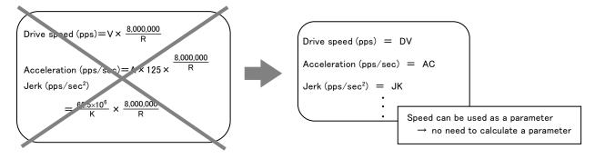
Fig. 1.1-8 Speed Parameter Setting
