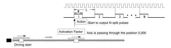
Fig. 2.6-3 Example 3 of Synchronous Action
