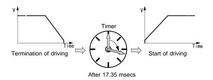
Fig. 2.9-4 Example 1: Timer Operation
