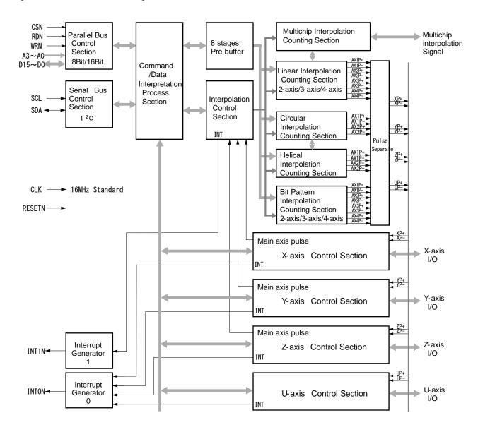
Fig. 1.2-1 MCX514 The Whole Functional Block Diagram
