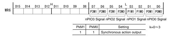
2 bits of WR6 register corresponding to the nPIOm signal that is used must be set to 1, 1 for the synchronous pulse output. For instance, when using XPIO2 signal, set D5, D4 bits (P2M1, P2M0) of WR6 register to 1, 1 and then write PIO signal setting 1 command (21h) with X axis into WR0 register.
