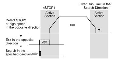
inactive. When nSTOP1 signal becomes inactive, the function executes Step 2 normal operation from the beginning.
