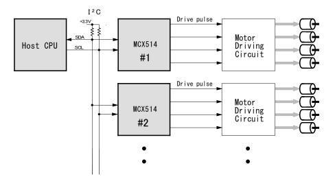
Fig. 1.1-14 I<sup>2</sup>C Serial Interface Bus
