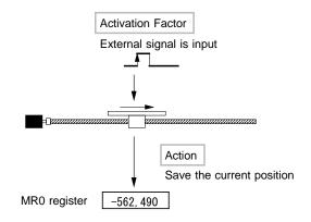
Fig. 2.4-3 Usage Example of Saving Parameters
