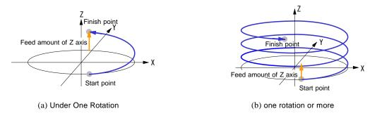
Fig. 3.3-4 The Feed Amount of Z/U axis
