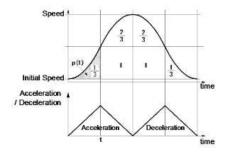
Fig. 2.2-9 The Rule of 1/12 of S-curve Acceleration / Deceleration
