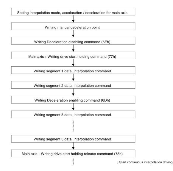
In this case, please note the manual deceleration point is the value for the output pulses of the main axis that are counted from the start of the segment 3.
