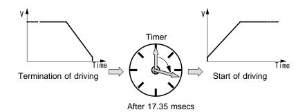
Fig. 2.9-1 Example 1 of Timer Operation
