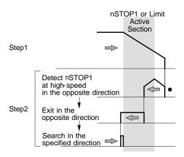
Fig. 2.5-8 Irregular Operation ④ of Step 2
