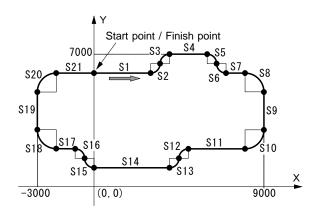
Fig. 3.7-2 Example of Continuous Interpolation
