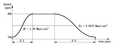
Fig. 2.2-15 Example of Non-symmetry S-Curve Acceleration/Deceleration Driving
