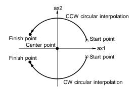
Fig. 3.2-1 CW/CCW circular interpolation
