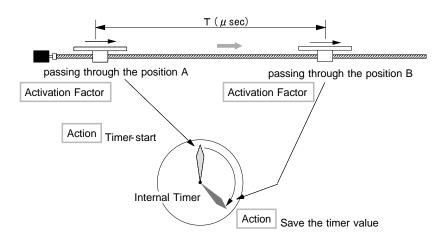
Fig. 2.6-9 Example 3: Synchronous Action
