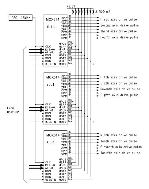
Fig. 3.10-1 The Connection Example of Multichip Axes Interpolation
