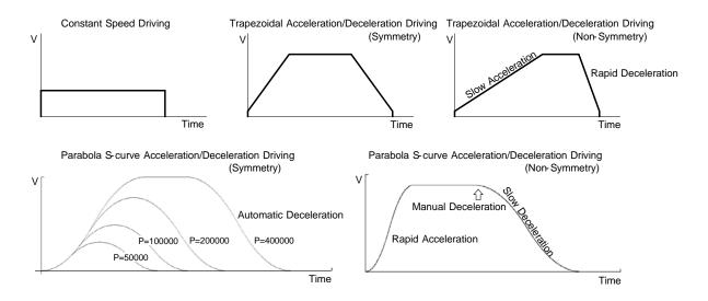
Fig. 1.1-9 Acceleration / Deceleration Drive Mode
