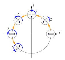
Fig. 1.1-2 Example of Normal Control of Z axis in XY axes Circular Interpolation
