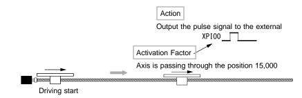
Fig. 2.6-8 Example 1: Synchronous Action
