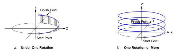
Fig. 1.1-1 Example of Helical interpolation
