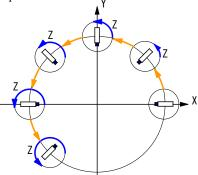
Fig. 3.3-3 Example of XY axes Circular Interpolation and Z axis Normal Control
