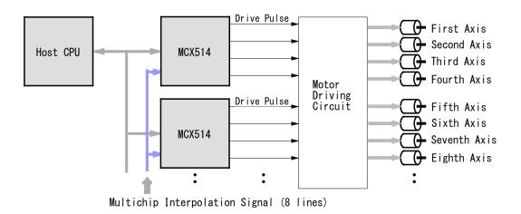
Fig. 1.1-4 Example of Multichip Interpolation
