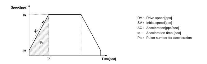
©Calculation Formula of acceleration AC when initial speed SV, drive speed DV and acceleration time ta are given
