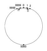
Fig. 2.3-3 Operation of Position Counter Ring Maximum Value 9999
