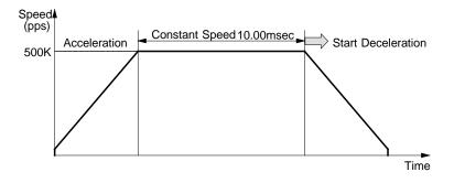
Fig. 2.9-3 Example 3 of Timer Operation
