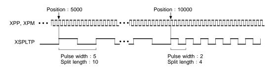
Fig. 2.7-6 Change Split Length and Pulse Width at Specified Position during the Driving
