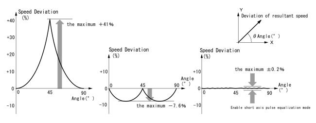
a. Constant vector speed: disabled b. 2-axis simple constant vector speed c. 2-axis high accuracy constant vector speed
