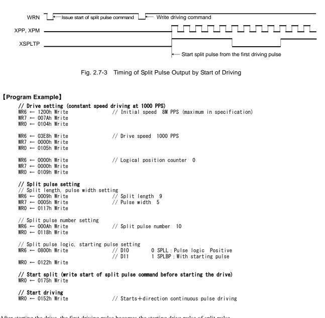
After starting the drive, the first driving pulse becomes the starting drive pulse of split pulse. After start of split pulse command is written, split pulses are not output unless driving starts, but D11 bit (SPLIT) of RR3 register Page1 becomes 1 at the timing of when start of split pulse command is written. ■ Example 2 Split pulse starts from position 5,000 in X axis.
