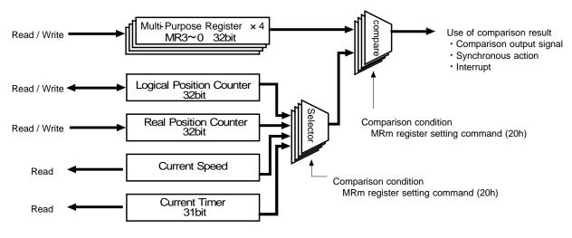
Fig. 2.4-1 Multi-Purpose Registers and Compare Function
