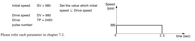
Fig. 2.2-2 Example of Constant Speed Driving
