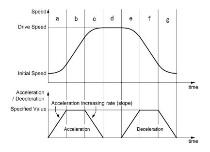
Fig. 2.2-12 Partial S-curve Acceleration / Deceleration Driving
