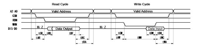
The figure shown above is used for 16-bit data bus accessing (H16L8 = Hi). For 8-bit data bus (H16L8 = Low), the address signals shown in the figure become A3 $\sim$ A0, and data signals become D7 $\sim$ D0.
