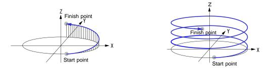
Fig. 3.3-1 Helical interpolation (under one rotation)
