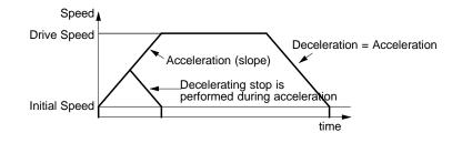
Fig. 2.2-3 Trapezoidal Driving (Symmetry)
