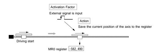
Fig. 2.6-2 Example 2 of Synchronous Action
