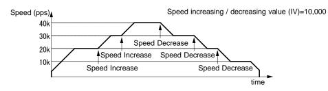
Fig. 2.1-12 Example of Speed Change by Speed Increase / Decrease Command
