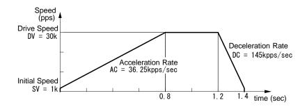
Fig. 2.2-6 Non-Symmetrical Linear Acceleration Driving (acceleration < deceleration)
