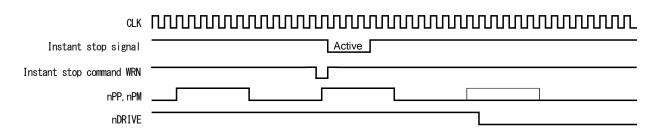
An instant stop input signal requires a pulse width of 2 CLK cycles or more even if the input signal filter is disabled. When the input signal filter is enabled, the input signal will be delayed according to the time constant of the filter.
