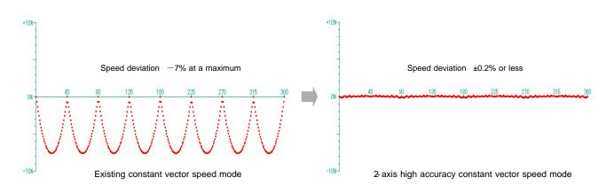
Fig. 1.1-6 Speed Deviation in Constant Vector Speed Mode
