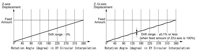
Fig. 3.3-5 Ideal Z-axis Feed in Helical Interpolation
