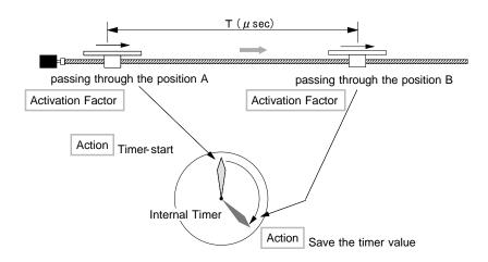
Fig. 2.6-4 Example 4 of Synchronous Action
