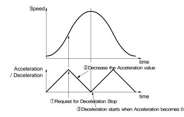
Fig. 2.2-10 Triangle Prevention of S-curve Acceleration / Deceleration by Decelerating Stop
