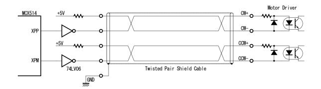
For drive pulse output signals, we recommend the user to use twisted pair shield cable due to the concern of EMC.
