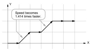
Fig. 3.5-1 Example of 2-axis Interpolation
