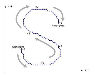
Fig. 3.4-1 Example of Bit Pattern Interpolation
