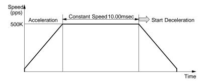
Fig. 2.9-6 Example 3: Timer Operation
