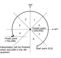
Fig. 3.2-5 CW/CCW Circular Interpolation
