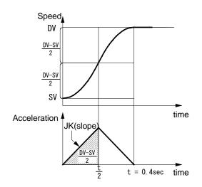
Fig. 2.2-11 Example of Symmetry S-Curve Acceleration / Deceleration Driving
