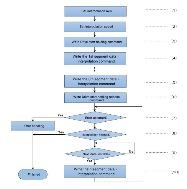
Fig. 3.7-1 The Flow of Continuous Interpolation
