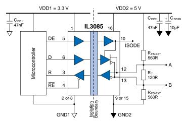
Figure 1c. Typical wide-body connections.
