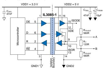
Figure 1a. Typical QSOP transceiver connections.
